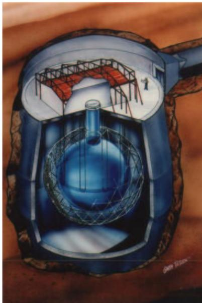
**Figure 5.4.** A schematic view of the SNO experiment. Courtesy of SNO.
